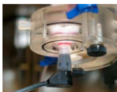
Fig. 5: Exposure to chemicals delivered 10 ul within a contact lens being mounted on a goldmann- tonometer head and with defined force exposed to the cornea mounted in the new culture chamber.
